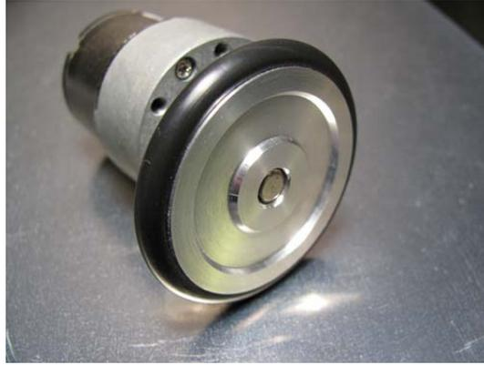
**Figure 4 Solid Rubber O-ring Used as a Tire for a Wheel**
