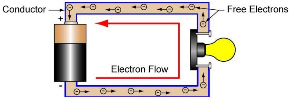
**Figure 20: Electron Flow – Current Flow from Negative to Positive**
