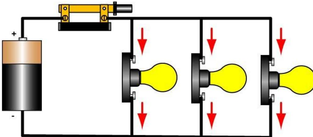
**Figure 23: Three Lamps in Parallel with Three Current Pathways**
