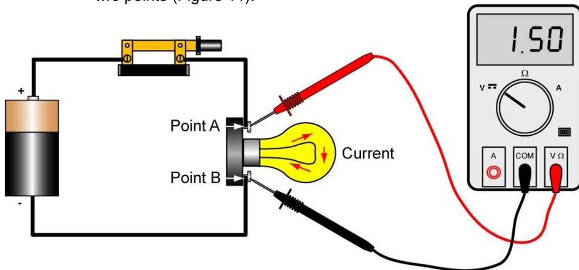
**Figure 11: 1.5 Volts Measured between Points A and B Drives the Current between those Points**
