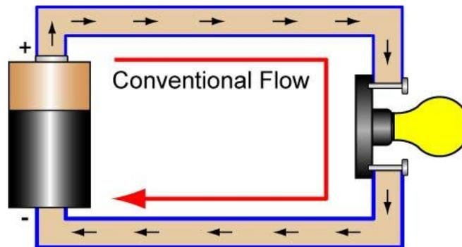
**Figure 21: Conventional Flow – Current Flow from Positive to Negative**
