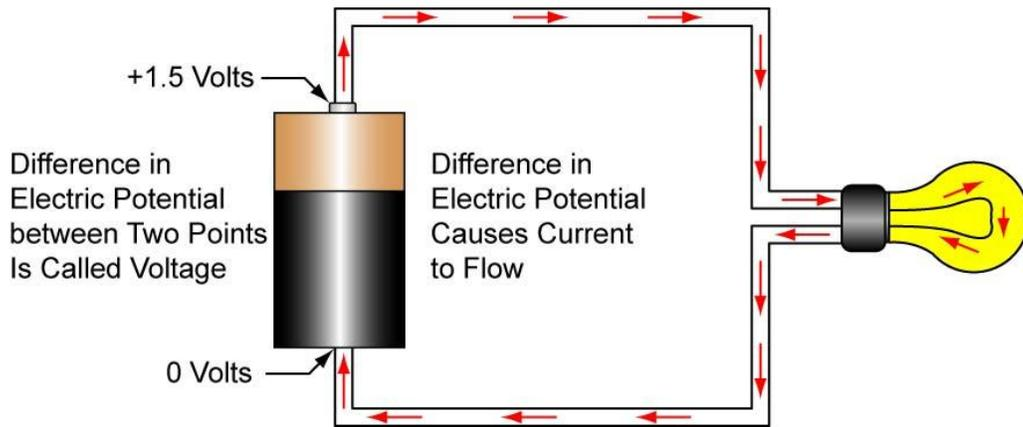
**Figure 3: Electric Potential Difference Causes Current to Flow**
