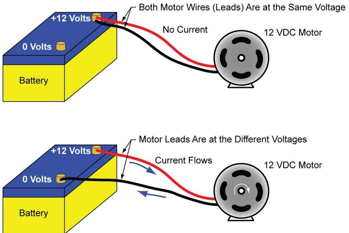
**Figure 13: A Difference in Voltage Creates Electrical Current through the Motor**
