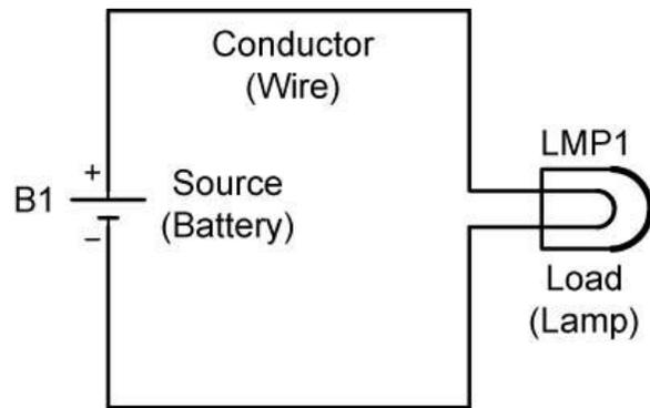
**Schematic of the Simple Circuit**
