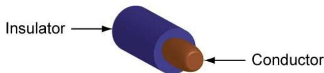
**Figure 17: Conductor and Insulator in a Wire**
