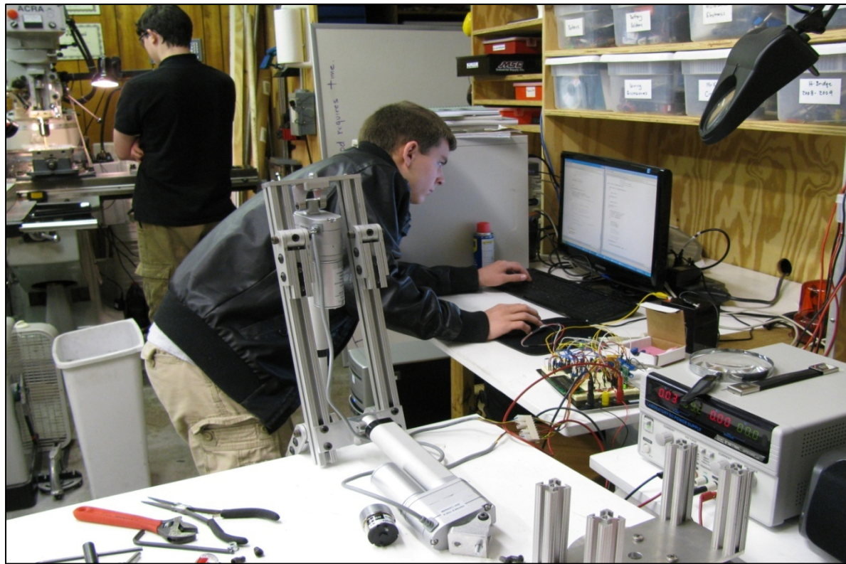
Image 5 (Above): Programming PIC Microcontroller To Control Linear Actuators. Image 6 (Below): Continuing Production Of The arm Using The Mill.
