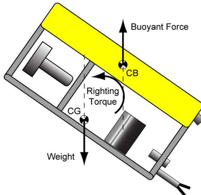
**Figure 17: Righting Torque Acting on a ROV which Is Out of Equilibrium**
