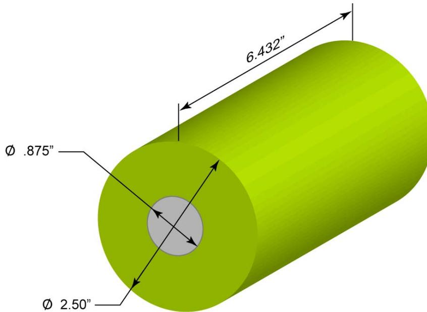
**Figure 3: Closed-Cell Foam Water Tube 6.432" Long**
