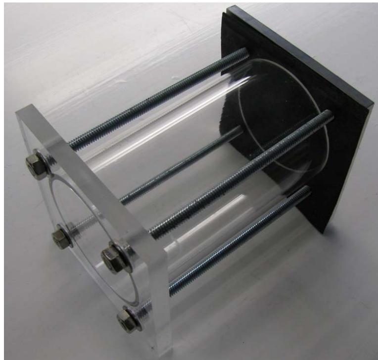
Final Assemble of the a Shortened Pressure Canister Housing
