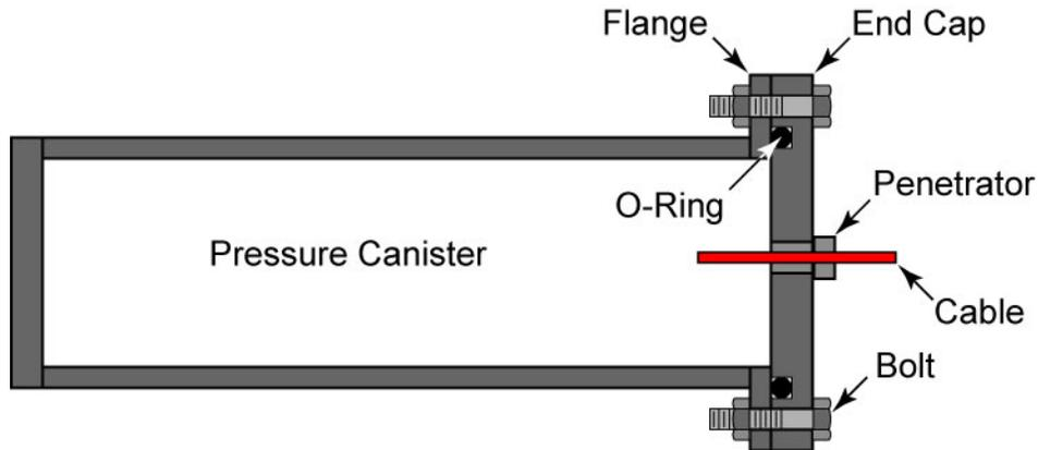
**Figure 8: End Cap Bolted to Pressure Canister Flange**
