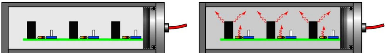
**Figure 12: Air Pressure Increased from Electronic Component Heating**
