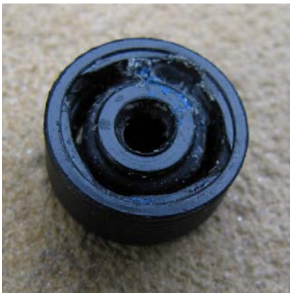
Figure 5a: U-Cup Seal
