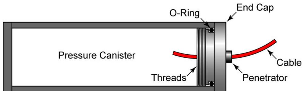
**Figure 10: Canister with a Threaded “Jam Jar” Seal**
