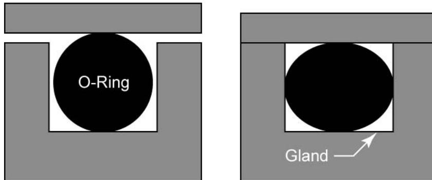
**Figure 4: O-Ring and Gland in a Static Seal**
