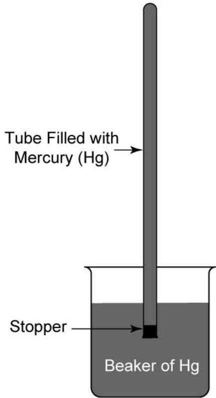
**Figure 10a:** A tube filled with mercury (Hg) is stopped with a cork and inverted into a beaker of mercury.
