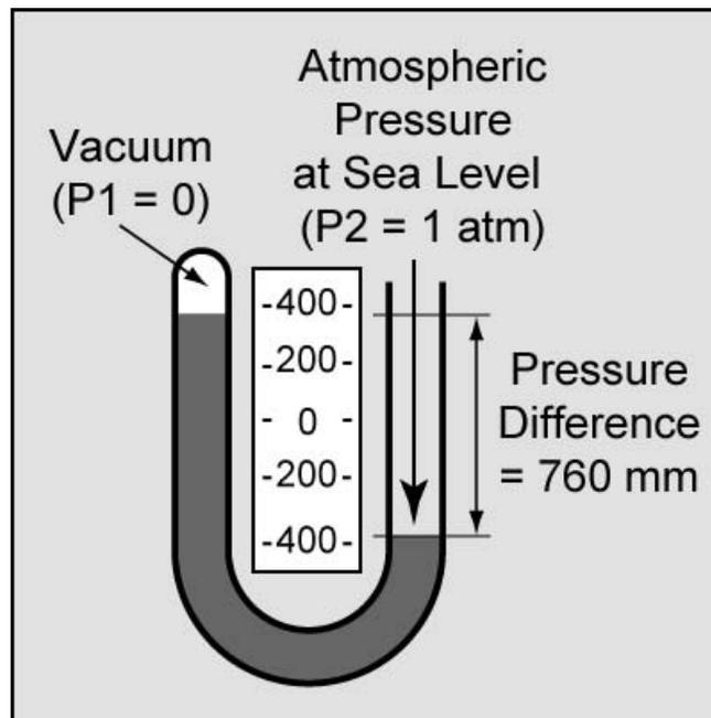
Figure 9: Barometer as an Adaptation of a Manometer
