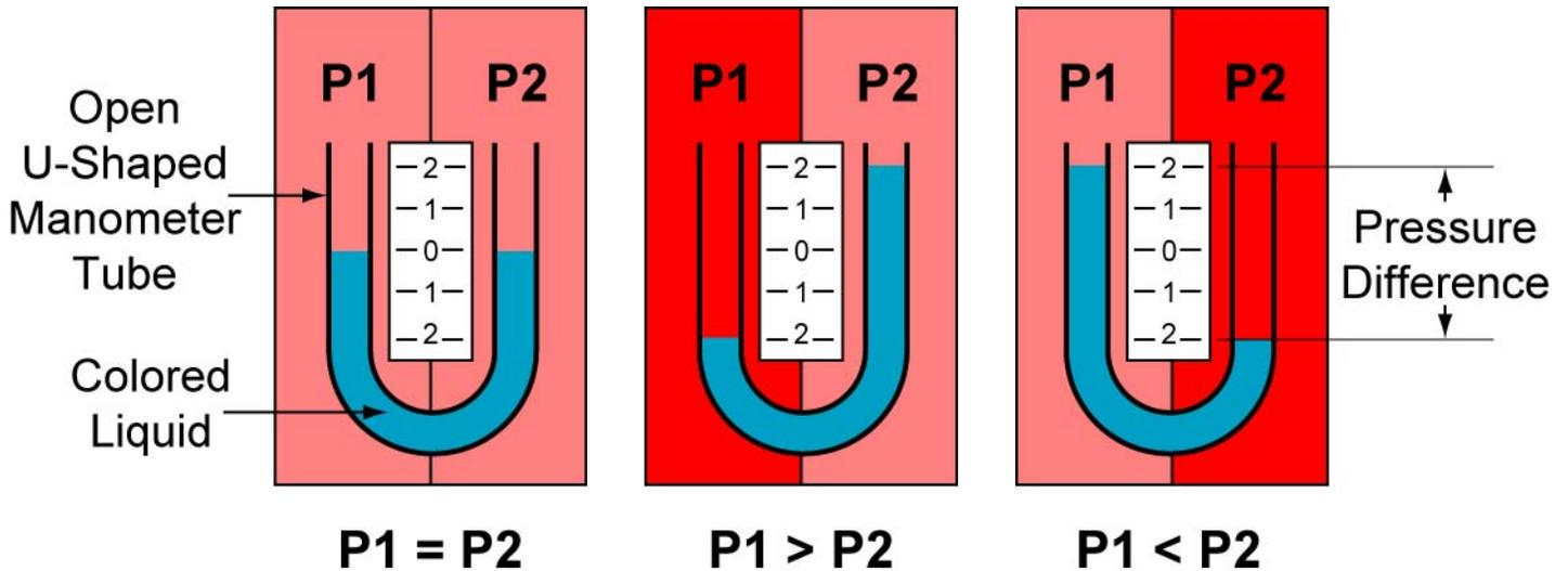
Figure 8: Manometer Responds to Fluid Pressure 1 (P1) and Fluid Pressure 2 (P2)
