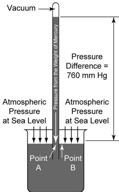
**Figure 10b:** When the cork is removed, mercury flows out of the tube until pressure due to the column of mercury at Point A just balances atmospheric pressure at Point B. The region above the mercury in the tube is an almost perfect vacuum with zero pressure. Therefore, the pressure of the mercury column at sea level equals the atmospheric pressure of 1 atm (760 mm Hg).
