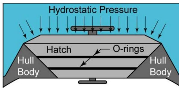
**Figure 17: Water Pressure Pressing Down to Help Seal Hatch**
