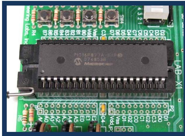
**Figure 3: 40-Pin PIC16F877A Microcontroller**
