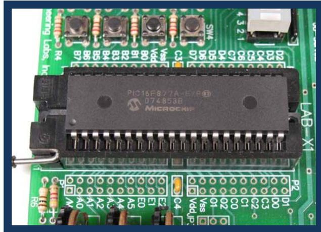
**Figure 2: 18-Pin PIC16F88 Microcontroller    Figure 3: 40-Pin PIC16F877A Microcontroller**
