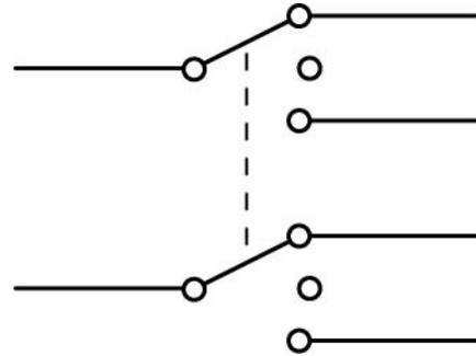
**Figure 13: Three Position DPDT with Central OFF Position**
