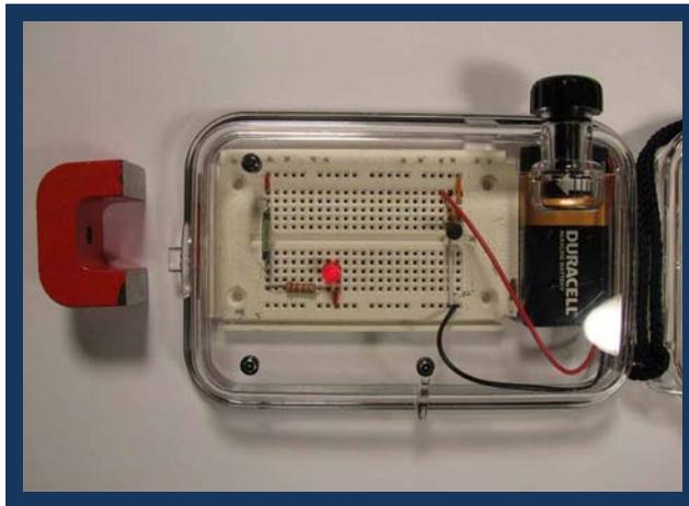
**Figure 7: Without any direct mechanical connection with the switch, the magnet closes the reed switch and the LED is illuminated.**
