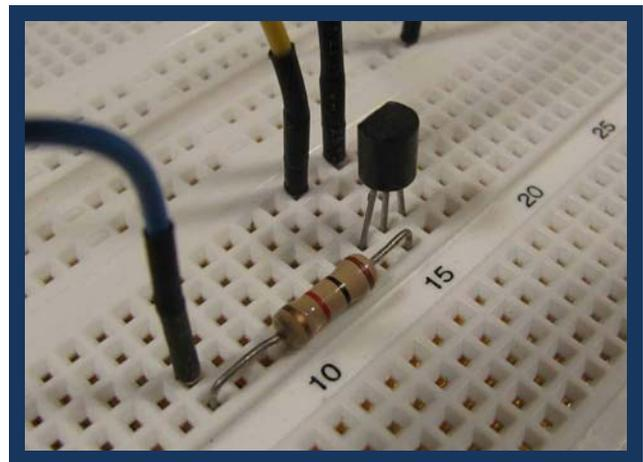
Figure 4: Transistor Switch
