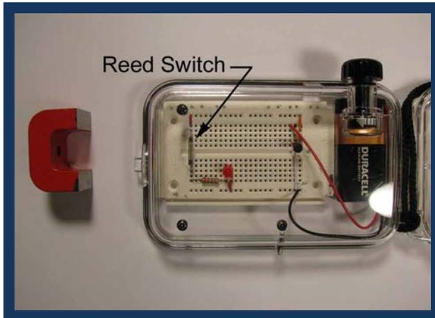
**Figure 6: The magnet is too far away to close the reed switch.**
