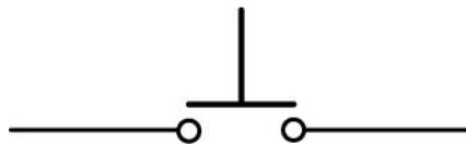
**Figure 14: SPST Normally Open (NO) Switch Symbol**
