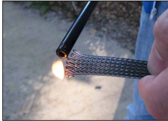
Figure 23: Fuse Filament Ends with Small Flame
