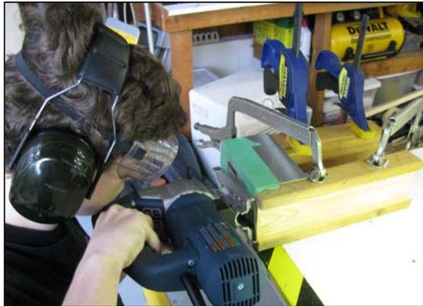
**Figure 6: Cutting the Square Hole with a Jigsaw**
