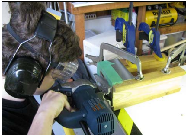
Figure 6: Cutting the Square Hole with a Jigsaw
