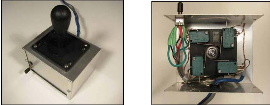
**Figure 7: Joystick Attached to the Aluminum Enclosure**
