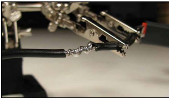
Figure 16: Soldered Black Wires and Heat Shrink Tubing Applied
