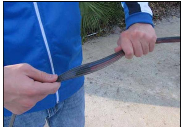
**Figure 25: Pushing Sleeving over End**
