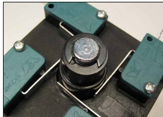
Figure 4: Holding down the Plastic Insert and Retaining Ring Inserted
