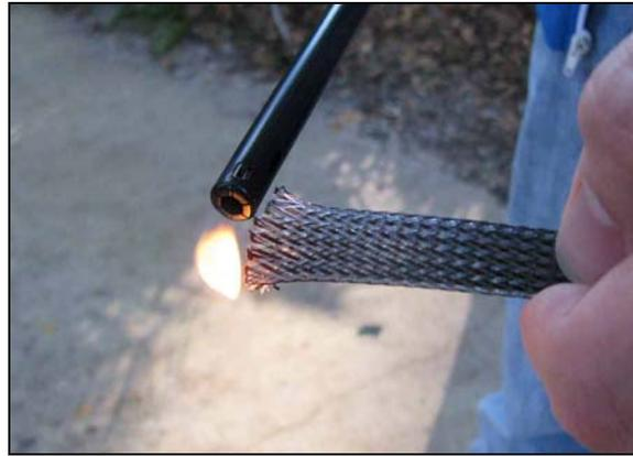
**Figure 23: Fuse Filament Ends with Small Flame**
