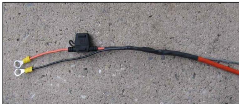
**Figure 17: Completed Power Connection**
