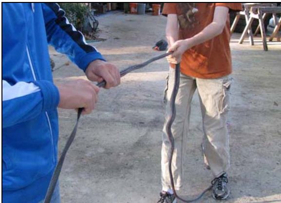
Figure 26: Work the Sleeving Down the Tether
