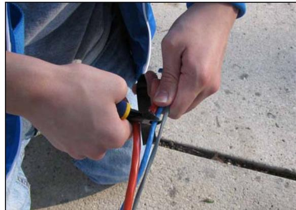
**Figure 20: Cut Three Cables to the Same Length**
