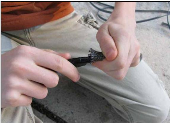
**Figure 24: Feed Sleeving over the Cables**
