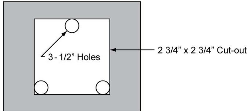
**Figure 5: Square Hole and 1/2" Hole Layout**
