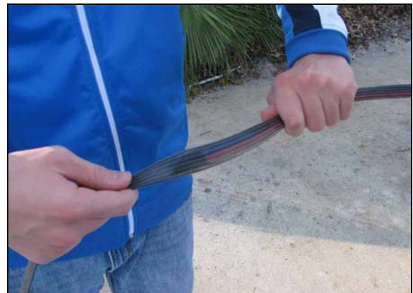
Figure 25: Pushing Sleeving over End
