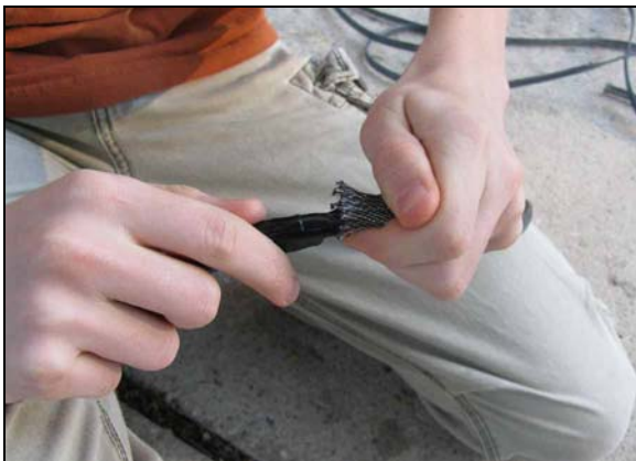
Figure 24: Feed Sleeving over the Cables
