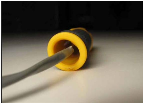
**Figure 12: Stripping the Outer Jacket from the 16/3 AWG Cable**
