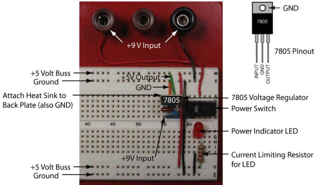
**Figure 26: A 7805 Fixed Output Voltage Regulator Circuit on a Solderless Breadboard**
