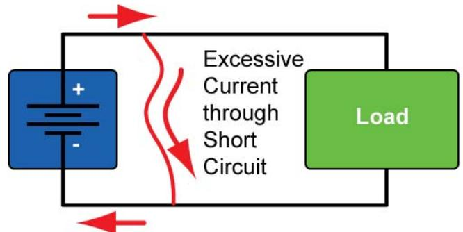
**Figure 17: Excessive Current through a Short Circuit in an Unprotected Circuit**
