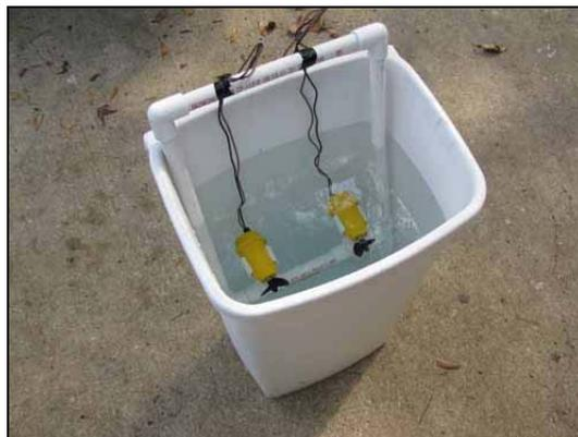
**Figure 3: Bilge Pumps Ready for the Test**
