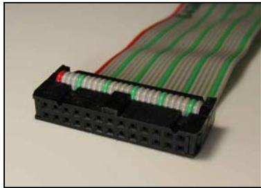
Figure 34: [Ribbon Wire Connector](#)
