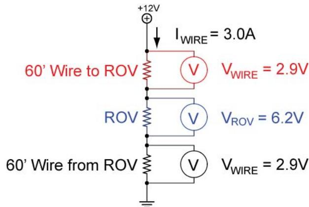
Figure 23: Schematic of Voltage Drops in 60' #22 Wire Tether
