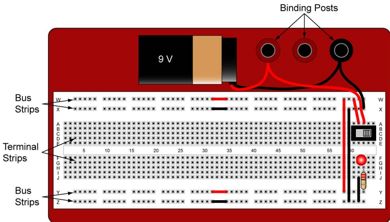
**Figure 27: Solderless Breadboard Set-up with +9V Supply Bus**
