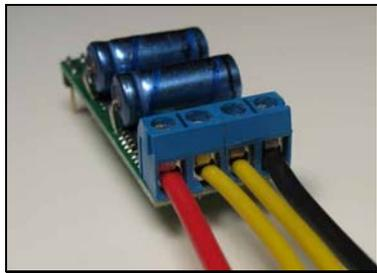
Figure 32: [PCB Terminal Blocks](#)
