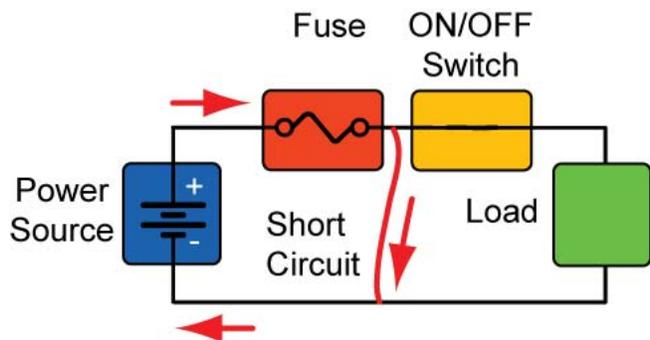
**Figure 19: At the instant a short circuit occurs, the excessive current flows through the fuse.**
