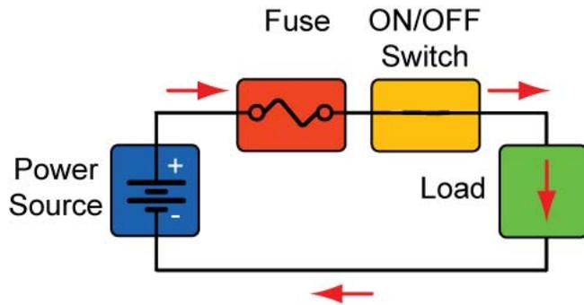
**Figure 18: Current flows through the load in a circuit that is protected by a fuse.**
