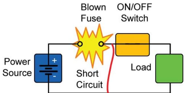
**Figure 20: The excessive current melts the fuse wire inside the fuse housing which opens the current path, stopping current flow.**
