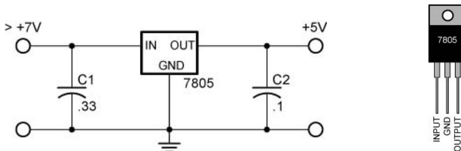
**Figure 25: Fixed Output Voltage Regulator Schematic and a 7805 Voltage Regulator in a TO-220 Package**
