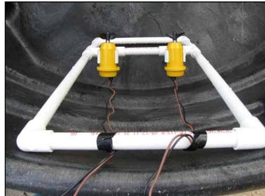
**Figures 1 and 2: Bilge Pumps Mounted to a PVC Frame**
