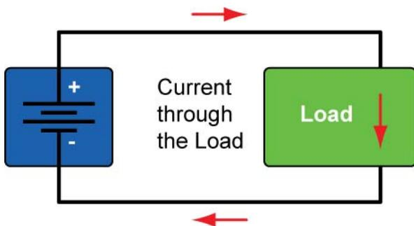
**Figure 16: Current through the Load (Its Normal Flow) in an Unprotected Circuit**
