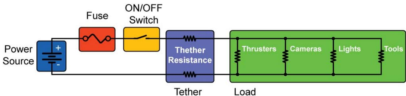
**Figure 13: Major Components of a Vehicle's Electrical System**
