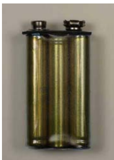
Figure 3: 6 – 1.5 Volt Cells Are Connected in Series to Form a 9 Volt Battery
