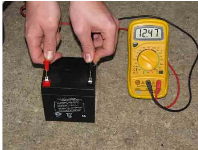
Figure 6: Checking the No-Load Voltage of a Battery
