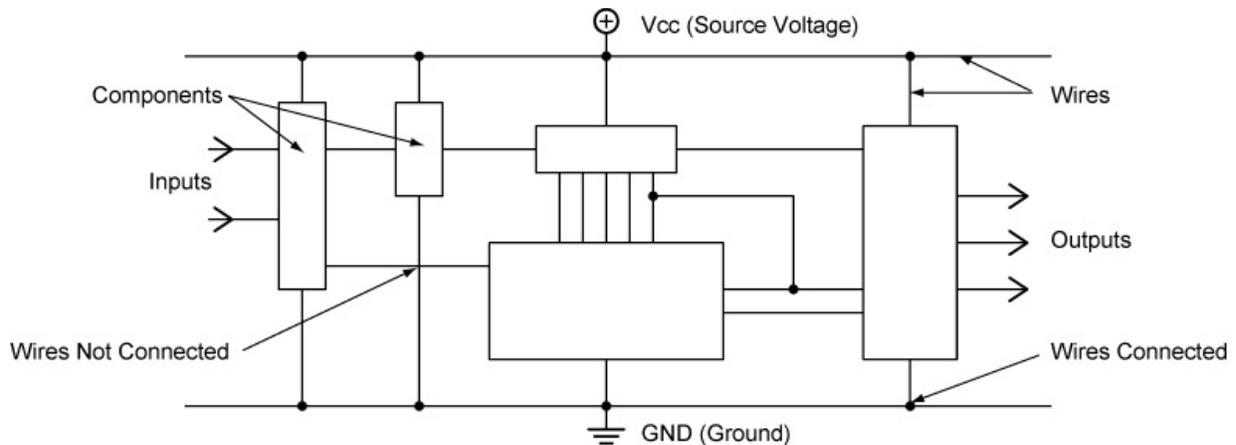
**Figure 18: General Layout of a Schematic Drawing**
