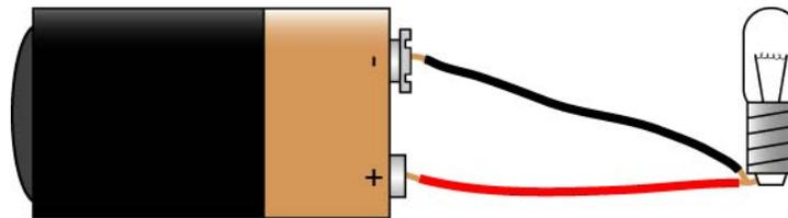
**Figure 13: Short Circuit**
