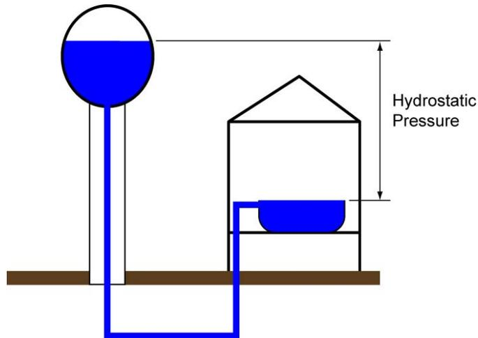
**Figure 4: Water Pressure from a Water Tower**
