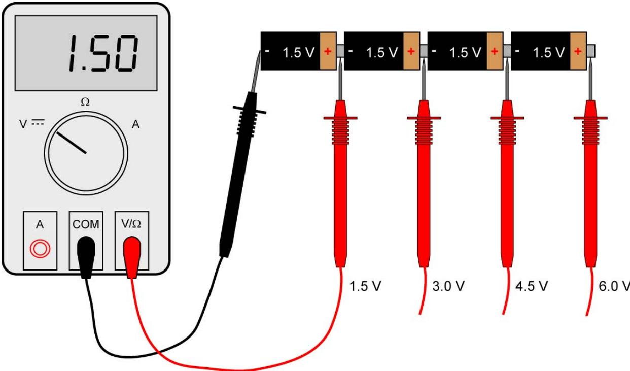
Figure 23: Voltages Add when Batteries Are in Series
