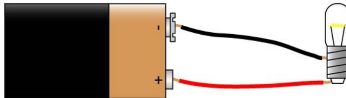
**Figure 12: Closed Circuit**
