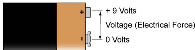
**Figure 5: Voltage (Electrical Force or Pressure) From a Battery**
