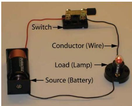
Figure 9: Simple Circuit
