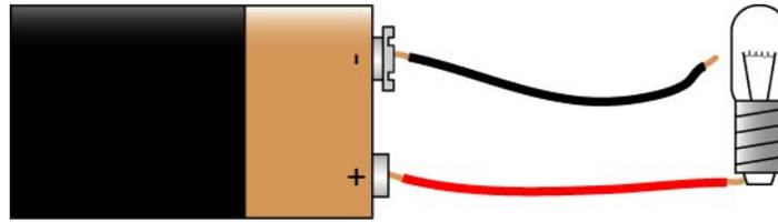
**Figure 11: Open Circuit**
