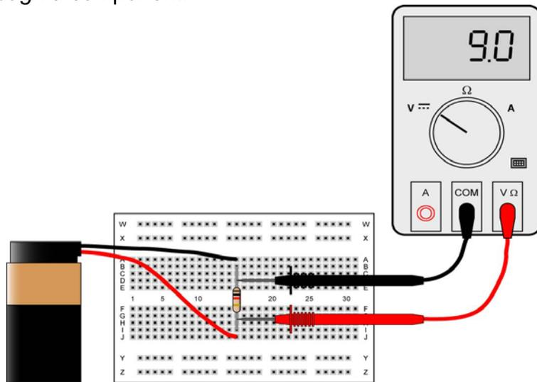
Figure 6: Measuring Voltage across a Component (Resistor)
