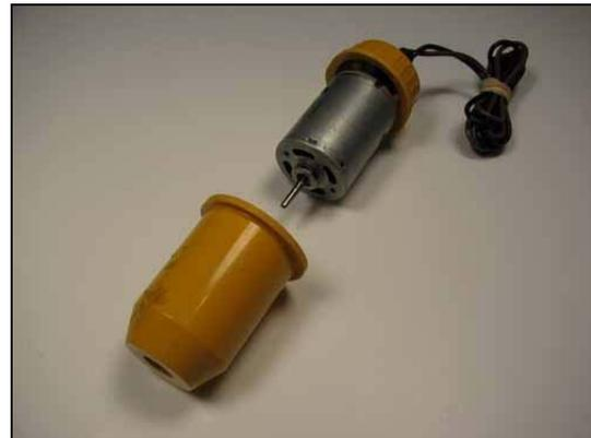
**Figure 5: Cutting Too Close to the Motor Breaks the Waterproof Seal**
