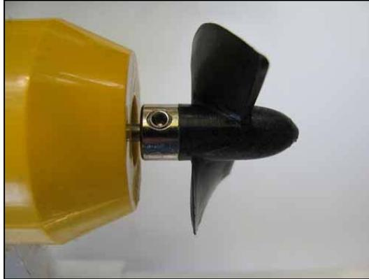
**Figure 9: Traxxis #1583 Propeller Attached to the Bilge Pump**
