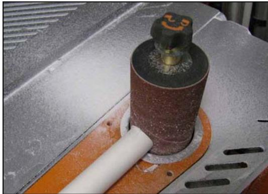
**Figure 12: Rounding the ½" PVC on a Spindle Sander**
