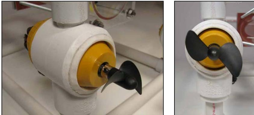
**Figure 10: Thruster Mount in Line with Frame Member**
