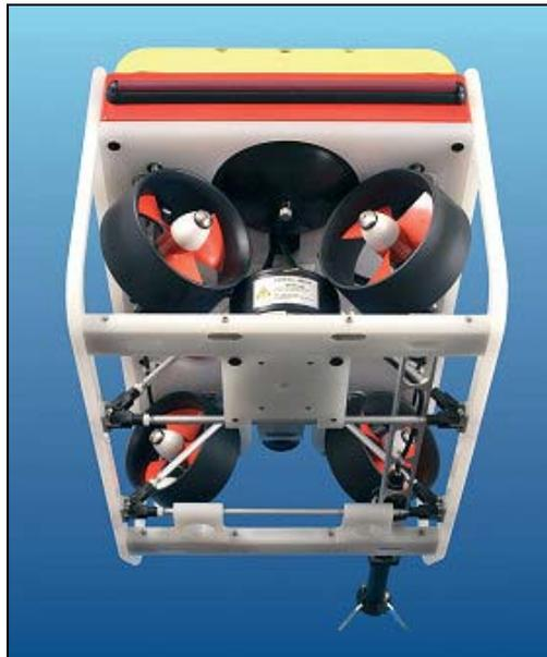
**Figure 15: Four Vectored Thrusters for Horizontal Movement**
