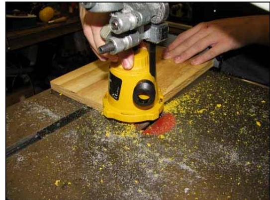
**Figure 4: Cutting Off the Housing from the Motor**
