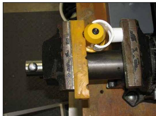
**Figure 8: Pressing the Bilge Pump into the Modified PVC Tee**
