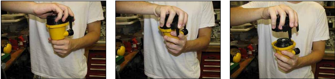
**Figure 1: Twist Bilge Pump Unit to Remove**
