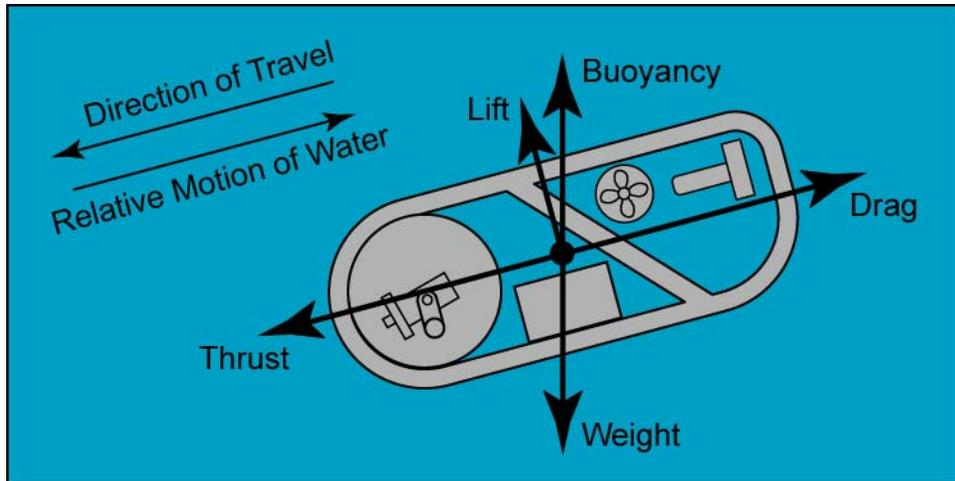
**Figure 9: Five Forces that Control a Moving Underwater Vehicle**
