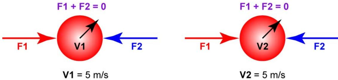
**Figure 5: If All the Forces Acting on an Object Are Balanced and the Object is in Motion, the Object Maintains the Same Speed and Direction over Time ( $V1 = V2$ )**
