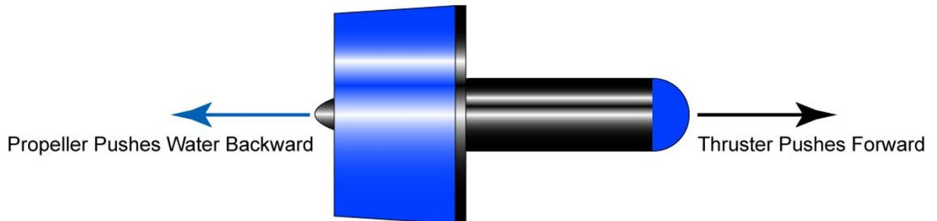
**Figure 8: Likewise, when a Thruster's Propeller Pushes the Water Backward, the Water Pushes the Thruster Forward**
