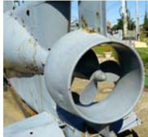
**Figure 20: Ducted Propeller**
