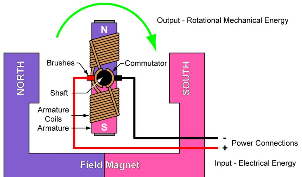
**Figure 13: Parts of a Basic Brushed DC Motor**
