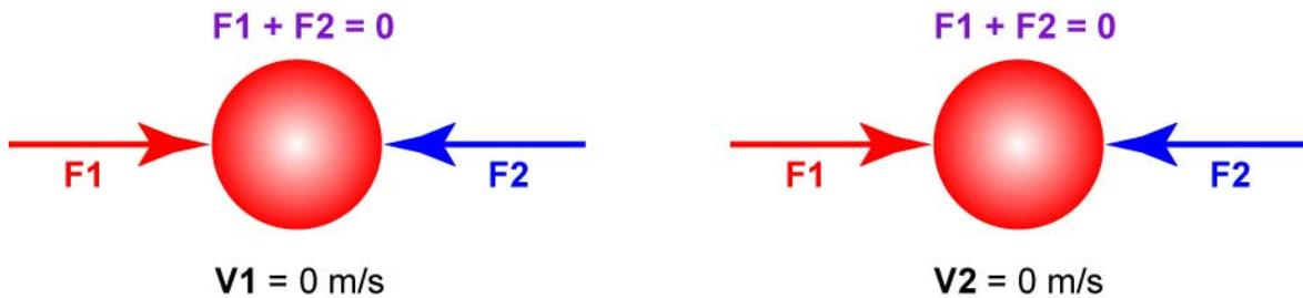
**Figure 4: If All the Forces Acting on an Object Are Balanced (Net Force = 0) and the Object is at Rest, then the Object Remains at Rest ( $V_1 = V_2 = 0 \text{ m/s}$ )**
