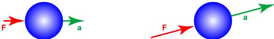
**Figure 6: The Larger the Force, the Larger the Acceleration**
