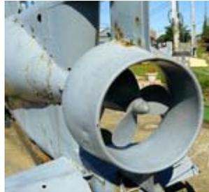
**Figure 20: Ducted Propeller**
