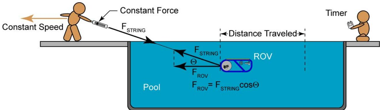
**Figure 12: Measuring Drag Empirically Using a Pull Type Spring Scale**
