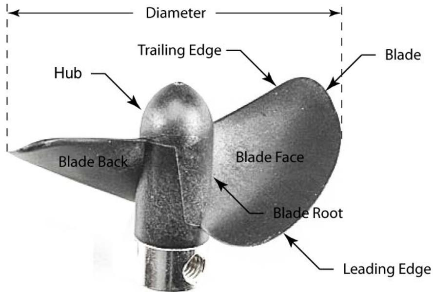
**Figure 17: Parts of a Right-Handed Propeller**
