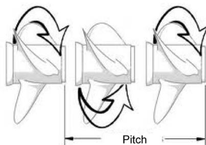
**Figure 18: The Pitch of a Propeller Making One Revolution**
