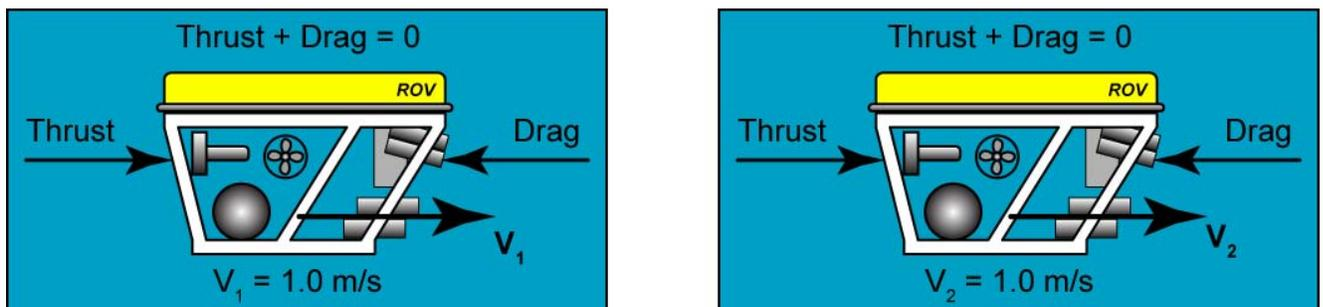
**Figure10: As in Figure 5, if All the Forces Acting on an ROV Are Balanced and the ROV is in Motion, the ROV Maintains the Same Speed and Direction over Time ( $V_1 = V_2$ )**
