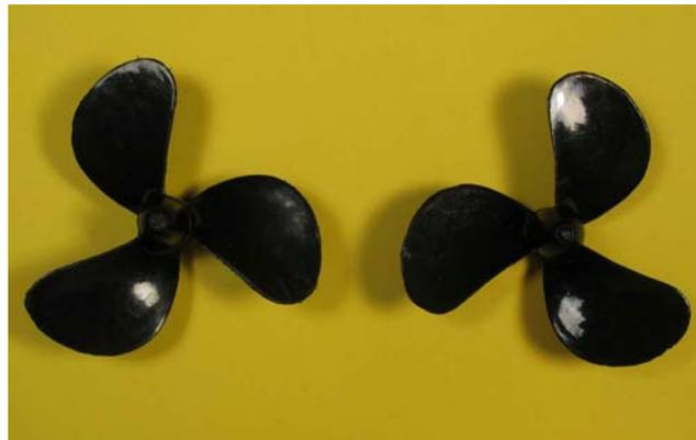
**Figure 19: Left-Handed and Right-Handed Propellers**
