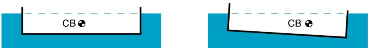
**Figure 10: As a Boat Pitches and Rolls, the CB Moves**
