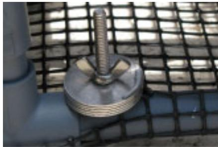
**Figure 3: Trim Post with Stainless Steel Washer Weights**
