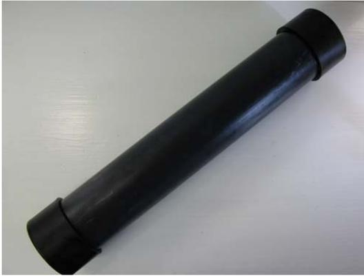
**Figure 19: Plastic Pipe Ballast with Glued End Caps**
