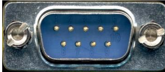
Figure 26-4: 9 Pin Connector on the PC – Male RS-232 DB9 Viewed from the Front
