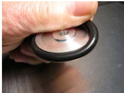
Install O-Ring Tread
