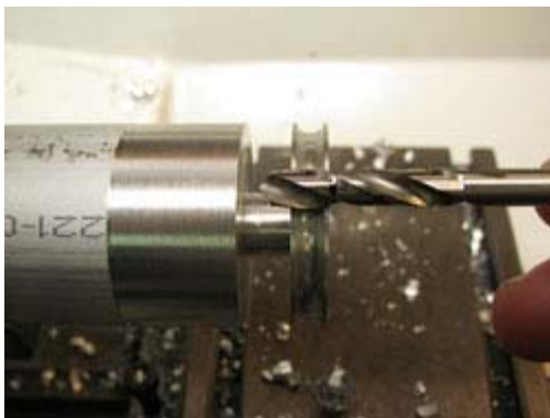
Mark the Bit for the Proper Depth
