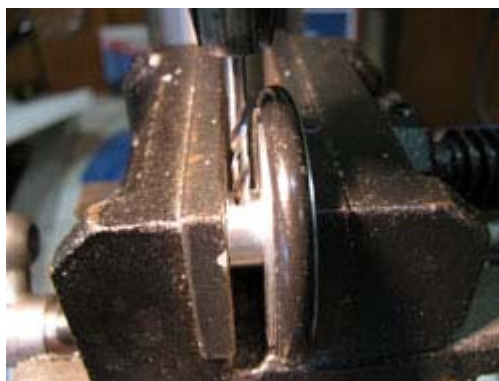
Drill Set Screw Hole
