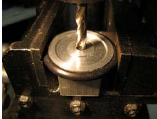
Finish Drilling Motor Shaft Hole
