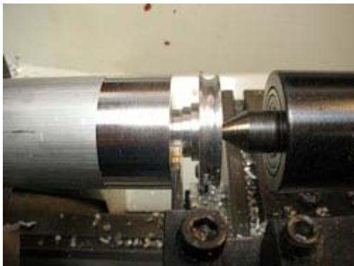
Nearing Completion of Notch
