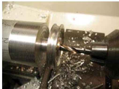
Drill Motor Shaft Hole
