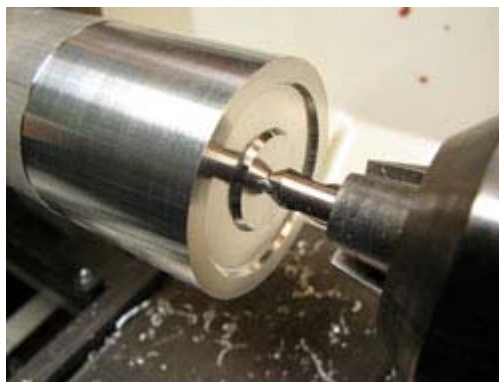
Center Drilling Face
