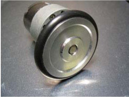
Finished Aluminum Hub with O-ring Tire
