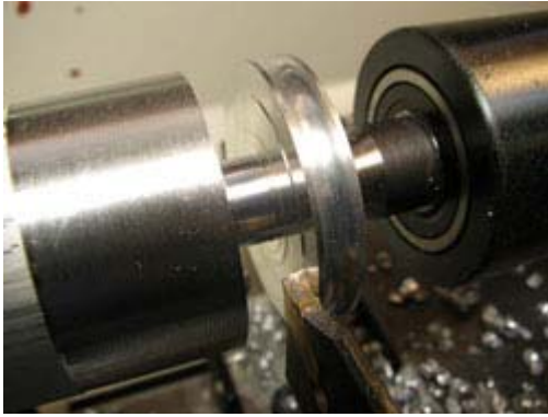
Facing the Inside of the Wheel
