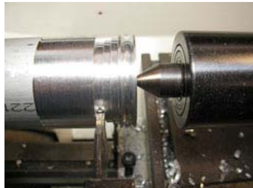
Turning Notch in Steps
