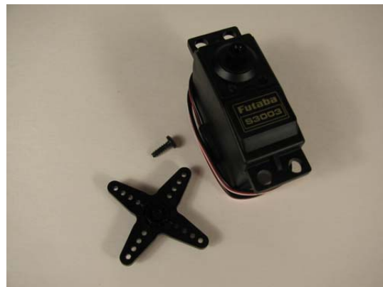
Remove Servo Horn
