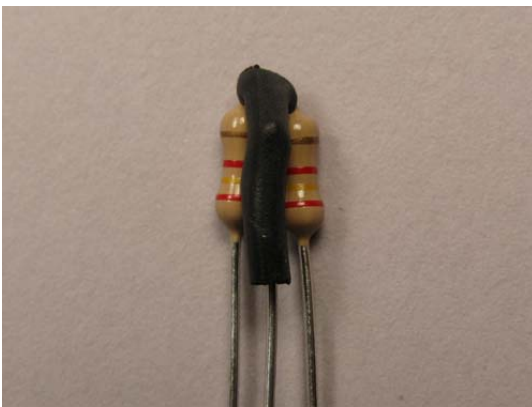
Install Heat Shrink Tubing
