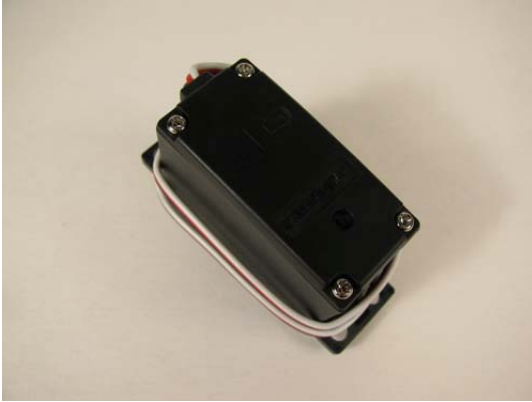
Four Rear Mounting Screws
