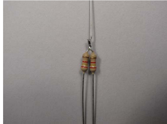
Solder Leads and Cut One Off
