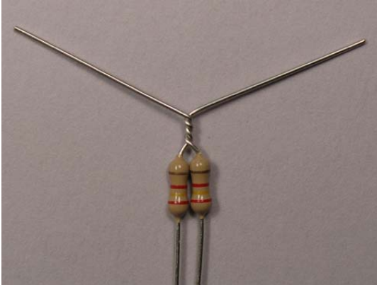
Twist Resistor Leads
