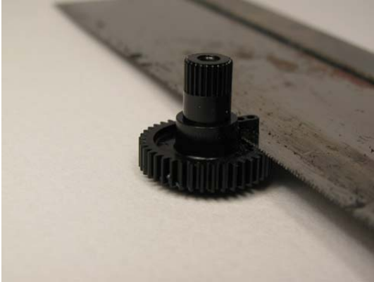
Cut Off the Potentiometer Stop
