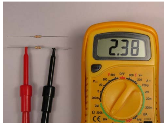
Measure and Match Resistors
