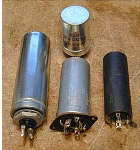
**Figure 4: Can Type Electrolytic Capacitors**
