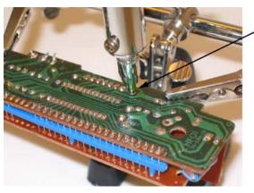
Insert the electric desoldering tool directly over the lead.
