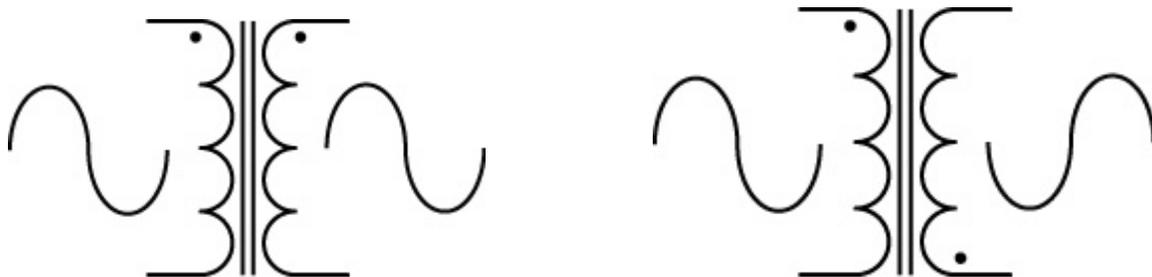
**Figure 32-10, Schematic Symbols Showing Dots and Polarity**
