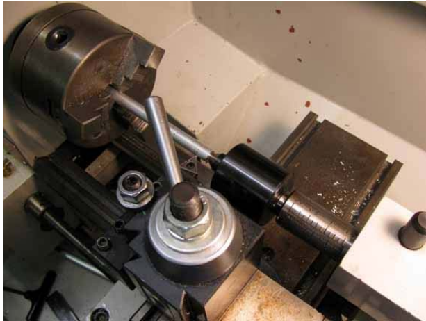
Rod and Live Center in Position
