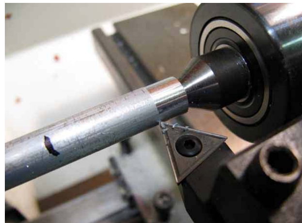
Milling the Rod to 32mm from the End
