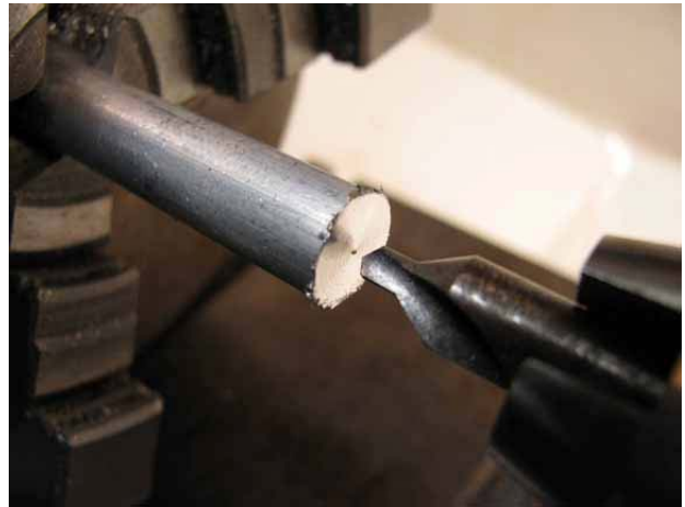
Center Drill in Position
