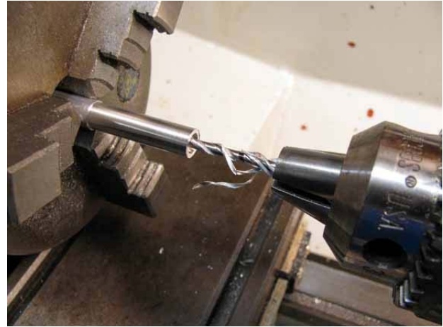
Drill to Mark on Drill Bit
