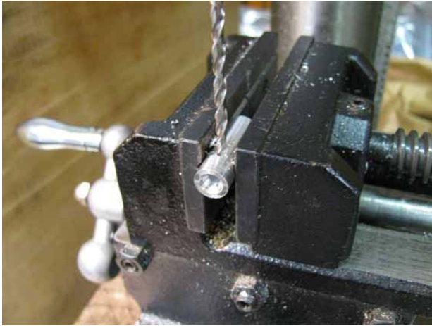
Drilling for Tap
