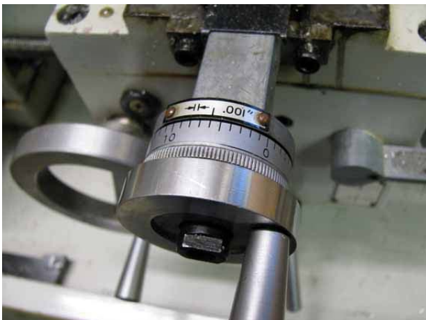
Handwheel Setting at 0.006"
