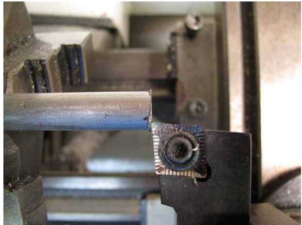
Position of the Diamond Insert
