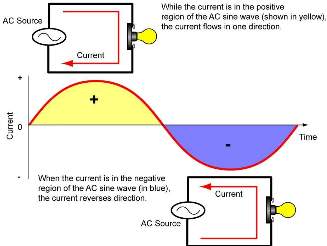
**Figure 19: Alternating Current Flows in Both Directions**
