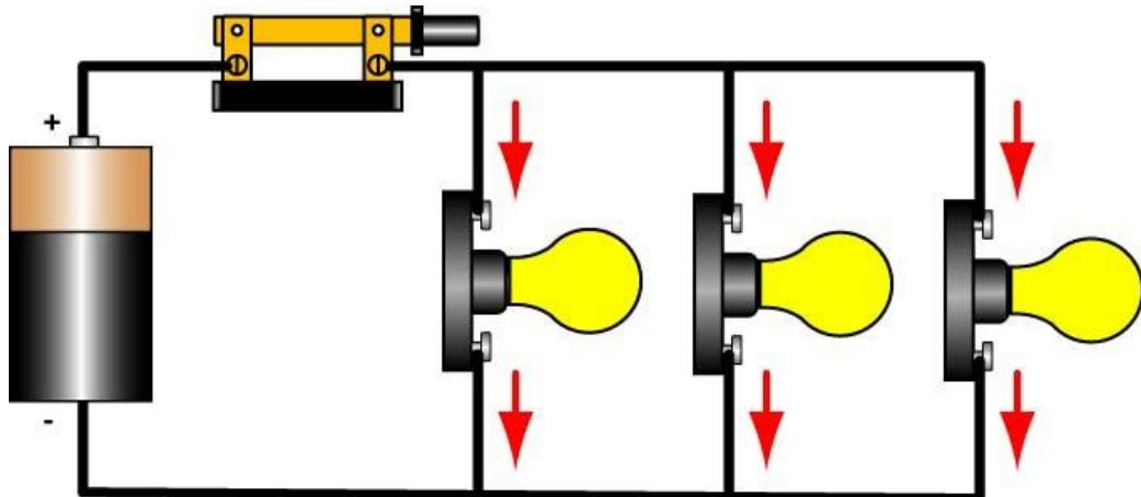
**Figure 23: Three Lamps in Parallel with Three Current Pathways**
