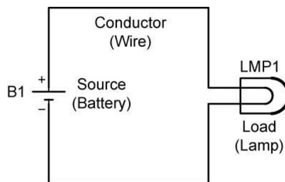
Schematic of the Simple Circuit
