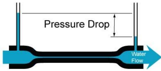
**Pipe with Severe Constriction and Pressure Drop**
