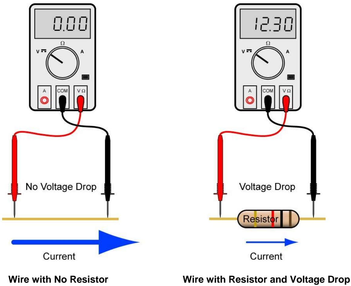
**Figure 16: A Resistor in an Electrical Circuit Reduces the Current and Produces a Voltage Drop across the Resistor**
