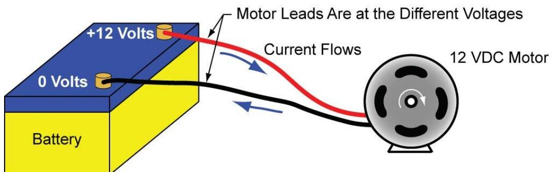
**Figure 13: A Difference in Voltage Creates Electrical Current through the Motor**
