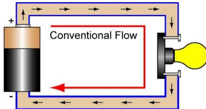
**Figure 21: Conventional Flow – Current Flow from Positive to Negative**
