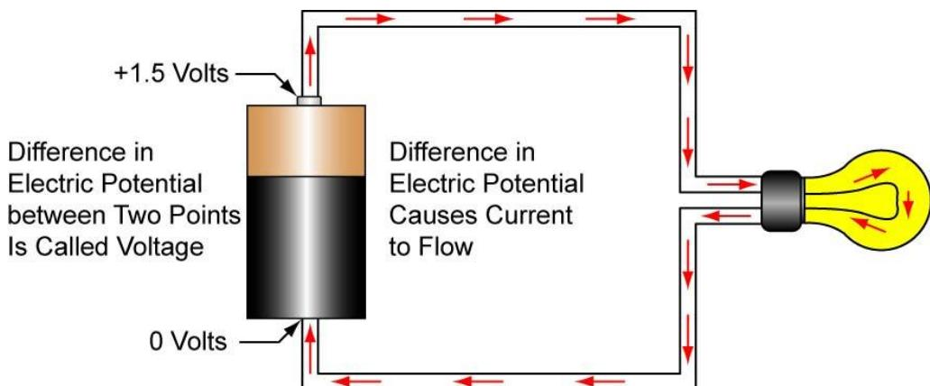
**Figure 3: Electric Potential Difference Causes Current to Flow**
