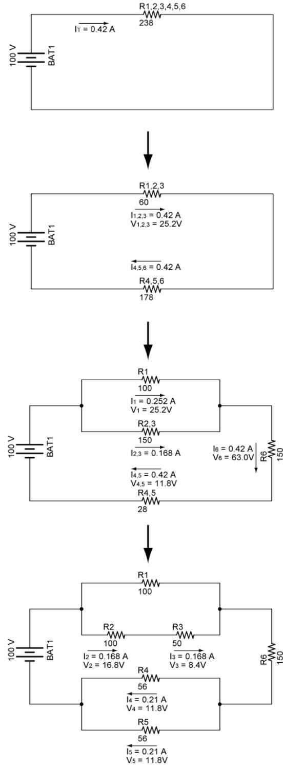
Figure 2 – Example of Contracting and Expanding a Combination Circuit
