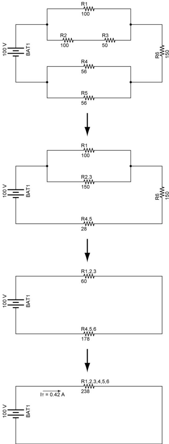
Expanding a combination circuit to determine the circuit currents and voltages:
