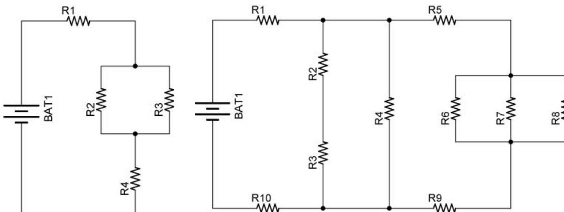
**Figure 1 – Examples of Combination Circuits**
