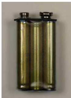
1.5 Volt Cells Are Connected in Series to Form a 9 Volt Battery
